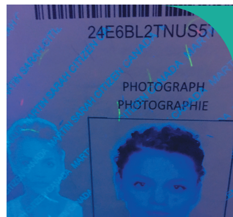
Critical data repeated in UV with biodata and portrait printed in UV blue and red. Embedded UV fluorescent fibres in multiple colours.
