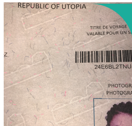
Emergency travel document (ETD) with colour inkjet print, machine readable elements, multi-coloured fibres and watermarks.
